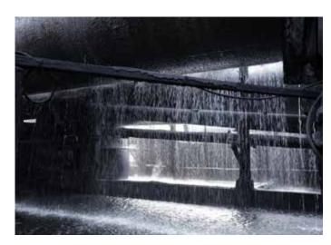
The bar leaves the quenching section for **Self Tempering** with the temperature of the core being higher than that of the surface. This allows heat to flow from the core to the surface, consequently tempering the surface, resulting in a structure called 'Tempered Martensite'. The core remains austenitic at this stage.
