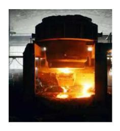
The unit was setup with 8x25 T, 11 MVA Induction Furnaces and a radial, 3 strand, 4/7 Met continuous caster producing  $100 \times 100$  mm size billets. Belt conveyors & bins installed for transfer & storage of DRI to SMS. Purchased pig iron (10%) and steel end cuts (20%) along with in house produced sponge iron (70%) melted. Ferro alloys added to obtain desired steel composition suitable for rebars.
