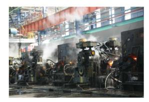
Thermo Mechanical Treatment - The Tempcore TMT online quenching process is adopted after rolling, with automated control of water pressure, nozzle angle and the rate of water flow. For Super Ductile rebars, it is very important to have a critical balance between chemistry and quenching parameters, essential in developing the desired properties.
